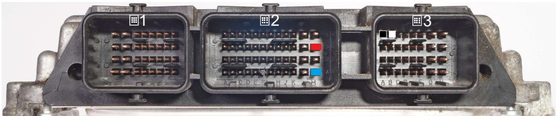
+12V | M2 | 2 | GND | M4 | 2 | CAN-H | A1 | 3 | CAN-L | B1 | 3 |
