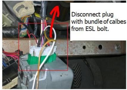
Connect emulator to bundle of cables in plug. ESL bolt leave unplugged.
