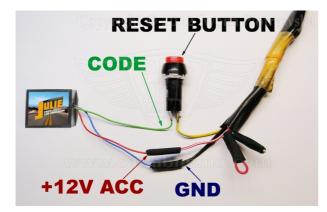
Connect code line by pressing the RESET button. In order to start the motorbike you first need to press and hold the RESET button, then turn the ignition and then release the RESET button. Now you can start the engine.
