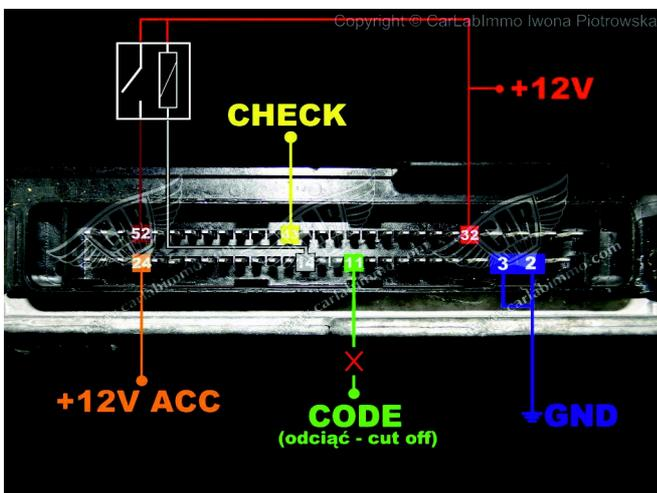
Cut off pin 11 from wiring in the car !!!
