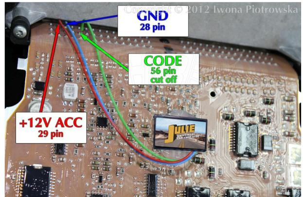
If you want to have engine diagnostics, DO NOT CUT pin 56 from the ECU. Instead, disconnect immobiliser or cut pin 10 of immo box.
