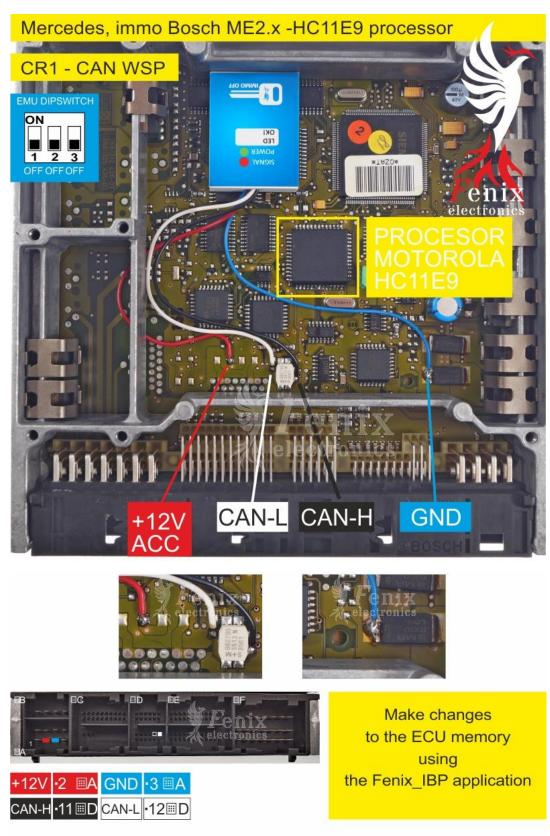
c. Controller Bosch z HC11E9 (320 6-cyl, 430 8-cyl)
