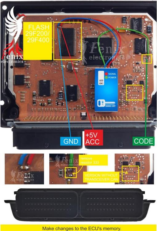
Read the memory. Make changes with the Fenix IBP application. Save the memory with the corrected file.
