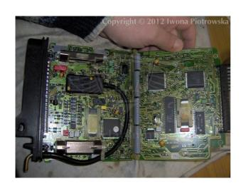
Connect immo line to pin 55. Disconnect immo. Connect A6 and A5 together.
