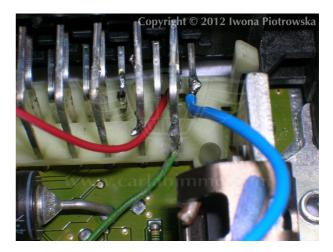
To have diagnosis, the immo line must be made in the reset button. Connect A6 and A5 together.
