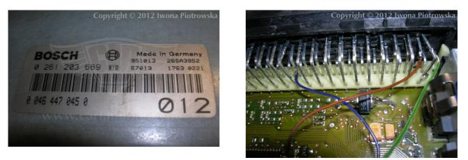
Connect immo line to pin 55. Disconnect immo. Connect A6 and A5 together. To have diagnosis, the immo line must be made in the reset button.
