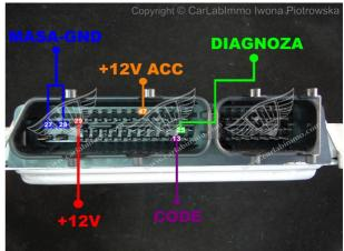
Cut off pin 13 from wiring in the car !!!
